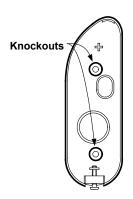
2 Replace the main unit onto the bracket.
