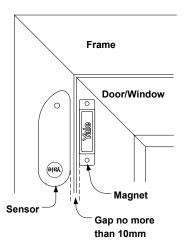
1 Find a location on the door/window where you would like the device to be mounted. The sensor should be on the frame while the magnet should be on the door/window. Once mounted make sure the tamper switch spring is fully depressed.
