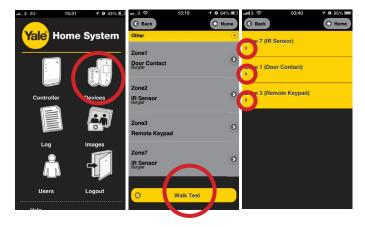
Hold the devices in the desired location and press the Test/Learn button (see below) on the accessories.
