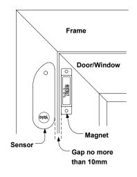
1 Find a location on the door/window where you would like the device to be mounted. The sensor should be on the frame while the magnet should be on the door/window. Once mounted make sure the tamper switch spring is fully depressed.
