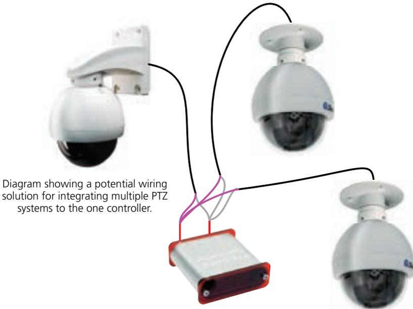
Diagram showing a potential wiring solution for integrating multiple PTZ systems to the one controller.
