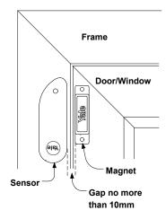
1 Find a location where the door/window contact is to be mounted. It should be mounted between the door/window frame and the door/window as shown at the top of the opening. The magnet is to go on the door/window while the sensor is to be placed on the frame. Windows can be protected in a similar way to doors. Make sure the tamper switch spring is fully depressed.
