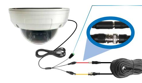
Connect the camera's DC and BNC socket cable to the extension cable's DC and BNC plugs
