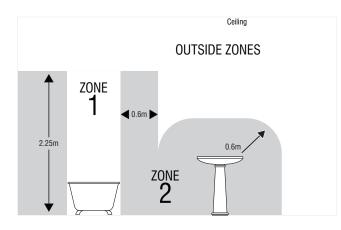
This product is suitable for use in Zone 2 and outside Zones of a bathroom. See diagram. If this unit is being fitted in a room containing a bath or shower, a 30mA RCD must be used - in accordance with IEE regulations.
