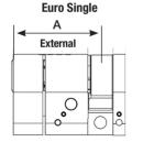
The Anti-Snap protection is on the external side of the cylinder. The first size on the product code indicates the external side.
