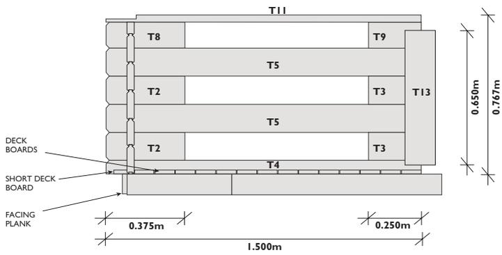
**NOTE:** BOTH TERRACE SIDES ARE CONSTRUCTED FROM THE SAME COMPONENTS
