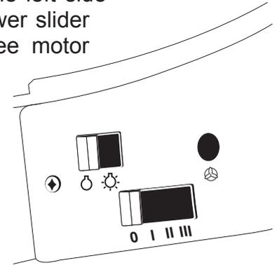
If the outer door is closed without switching off the fan motor, or lamps, an override switch will turn the cooker hood OFF. When the outer door is opened the cooker hood will resume working at its previous settings.
