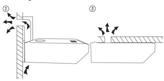
• The cooker hood can be either mounted on a wall (fig. ②), or underneath a suitable kitchen cabinet (fig. ③).
