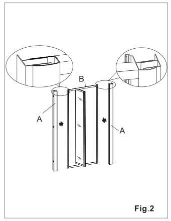
3a. Place the shower door on the shower tray, and position it so that there is an even gap of not less than 10-15mm to the front edge of the tray.
