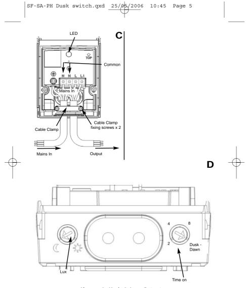
View on underside of unit shows adjustments
