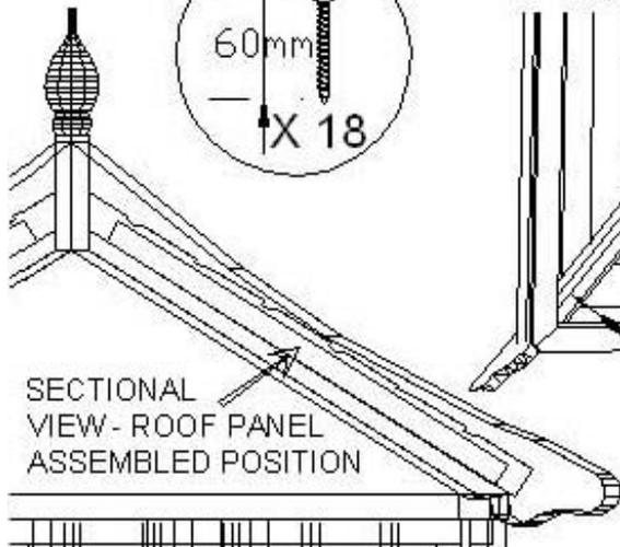
SECTIONAL VIEW - ROOF PANEL ASSEMBLED POSITION
