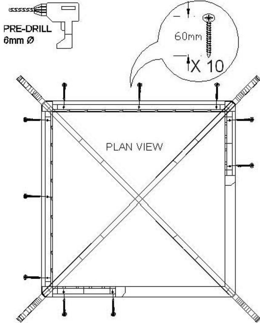
FROM ABOVE SCREW DOWN ROOF BRACES (L)
