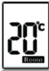
Pressing the temperature setting dial will allow the user to check the current room temperature which will be displayed for approx 7 seconds before returning to the set temperature.
