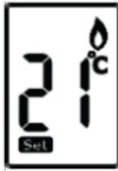
The display will show the required temperature setting and can be adjusted in increments of 1°C. To adjust the required temperature setting turn the dial anti clockwise to decrease it and clockwise to increase it.
