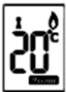
A radio mast symbol with no radio waves indicates that the thermostat has not been signed on to enable it to communicate with the timeswitch. In this case you may wish to contact the Installer as the indication is that the product has not been commissioned when the installation took place.
