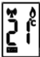
The aerial symbol complete with radio wave symbols in the display of the thermostat indicates that it is communicating satisfactorily with the timeswitch.
