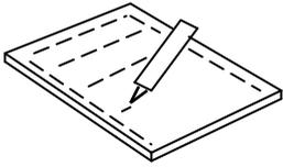
Apply a suitable adhesive to the rear surface of the splashback. Use a silicone, 'Grip Fill' or similar product.
