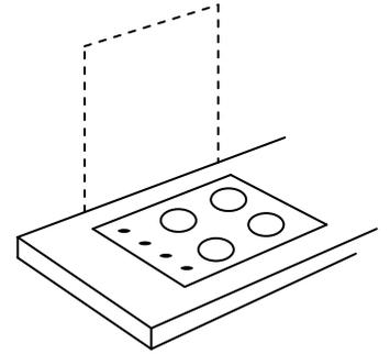
Apply the splashback to the wall and push firmly to the wall to ensure a good contact between the wall and the adhesive. Always refer to the adhesive manufacturers instructions regarding the length of time required for the adhesive to cure or dry. The splashback will need to be supported during this period to ensure it does not separate from the wall.
