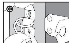
**Operation** - Slide flat plate into slot in chain anchor. When chain not in use place end ring on chain hook.
