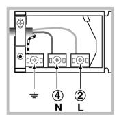
Voltage Frequency: 230 V-1+N 50Hz Fuse Section: 16A Supply cable: 3x1.5mm<sup>2</sup>
