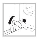
2. Use a screwdriver to lift up and turn the small levers **F** located on the two hinges (*see diagram*).
