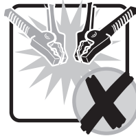
Anti-Arc Protection The battery clips will not spark if touched together.
