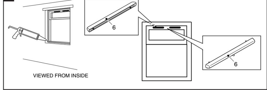
To ensure that the window operates smoothly it is vital that the frame is installed correctly. The frame **MUST** be fitted plumb and square. Check with a spirit level of adequate length, by measuring the frame corner to corner diagonally to achieve an equal measurement, or by using a square. It is also recommended that the window is checked for bowing by using a long straight edge.
