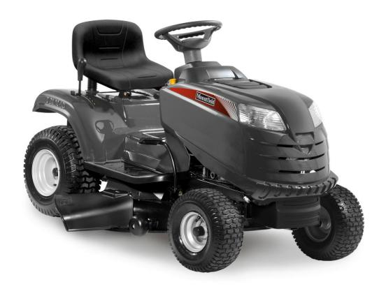
Mountfield's T38M-SD lawn tractor offers a highly effective solution if you don't want to collect your grass clippings as the twin bladed 98cm cutting deck can mulch or side discharge.
