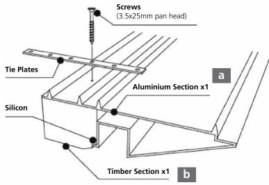
**Note:** Pilot Drill 2.5 x 25mm into underside of sill assembly, through the aluminium and into the timber, at positions 100mm, 250mm and 400mm from each end, then at no more than 400mm centres in between.
