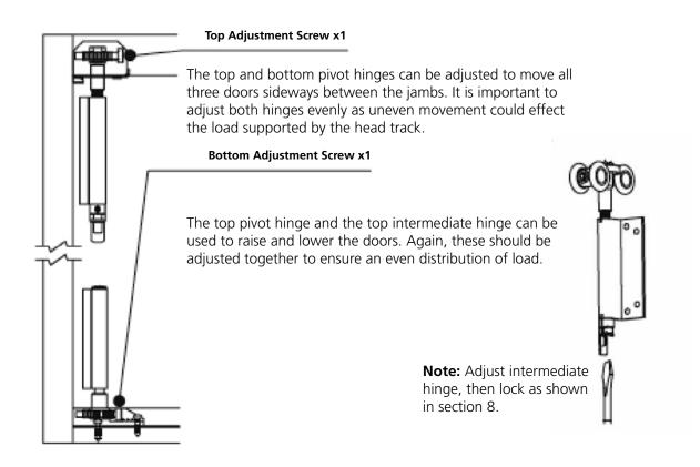
The doors should be adjusted so that there is an even gap at the head, sill and jambs. The nominal clearance at the head and sill is 5mm and that at the jambs is 8mm. If movement of the timber has occurred creating clearances greater than the target dimensions the gap at the multipoint lock should be altered by adjusting the pivot hinge(s) so that the latch engages correctly.
