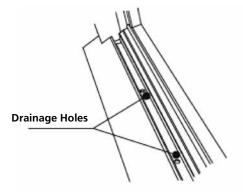
Check once more, that the jambs are vertical, that the head and sill are level and that the diagonals are within 5mm of each other.
