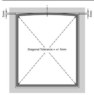
In order to produce a camber in the head track as shown opposite the fixings to the head need to be fitted in stages reducing the gap between the head and the supporting structure at each stage.
