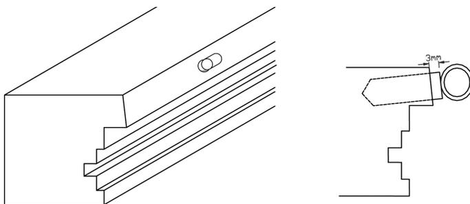
The deadbolt should be tapped into door stile to a minimum depth of 12mm, as shown in Fig 8.
