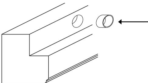
Top and bottom keeps must be fixed as in Fig 4.
