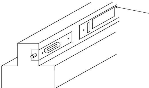
With the three hinges fitted locate the door into the frame jamb: at this point you may require assistance in holding the door while the hinge pins are inserted into the hinges. Do not insert the hinge pins fully until satisfied the door is hung correctly. Once this is done, close the door and engage both top and bottom shootbolts (G) in position.
