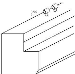
Tap deadbolt keeps in flush, or slightly below face of jamb rebate as in Fig 3.
