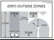
This product is specially designed for installation in a bathroom. It is IP65 rated and can be fitted in Zone 1, Zone 2 and Outside (dry) zones of a bathroom see diagram left. The bezel on this product provides the IP65 protection. The electrical parts of this product must be installed in a fully enclosed ceiling void with the bezel fitted to maintain the IP65 rating. Do not use the product without the bezel fitted.
