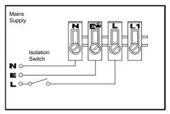
The diagram below also shows the required connections for the addition of slave luminaires. When adding slaves, be sure not to exceed the maximum switchable load (see Technical Specifications).
